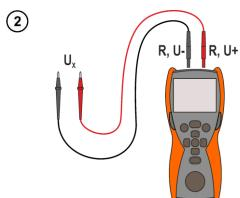
Connect the meter to a voltage source.
