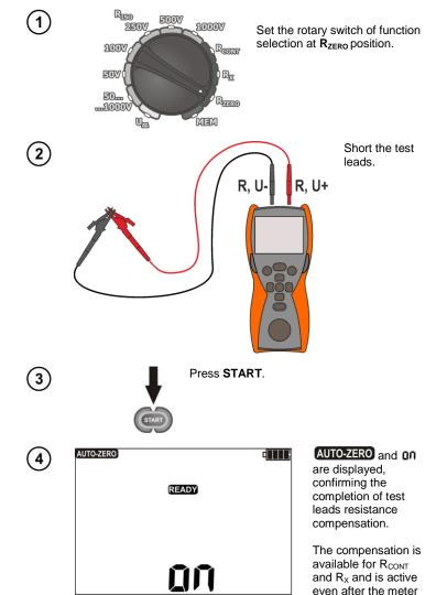
In order to remove the compensation made (and return to default calibration), perform the above-mentioned activities with test leads open – messages
