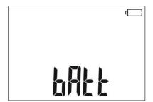
Batteries / rechargeable batteries fully discharged.
